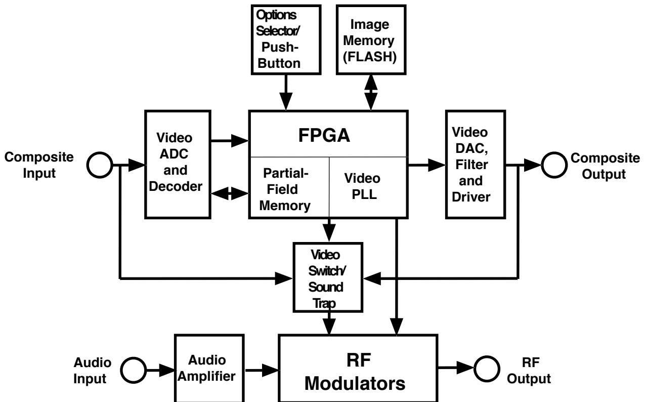
The incoming video is digitized and processed by the TVP5150A using a 14.318MHz reference crystal to the ITU-601 (formerly known as CCIR601) specification. All internal timing is generated using this crystal. The video is
